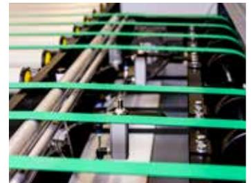
▲ PlateLink 46-XR has a simple belt drive configuration for easy and secure plate transportation.
