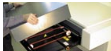
Removable top cover for easy access to belts, electronics etc.
