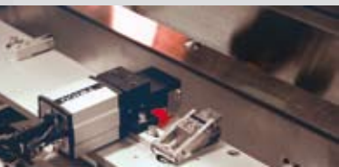
Vision registration Dual high-resolution CCD cameras register the plates with an accuracy of 0.02 mm (0.00078")
