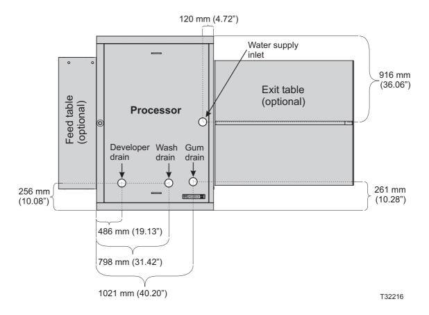
Prepare the installation site for water supply and drain connections according to the illustration above. Please also refer to the processor dimensions described earlier in this document.
