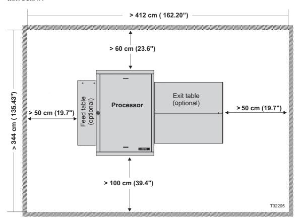
For CTP On-line processors the space requirements at the processor front has to be decided separately.
