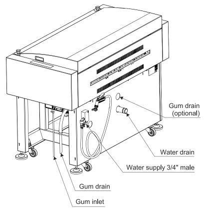
Prepare the installation site for water supply and drain connections according to the illustration. Please also refer to the "Space requirements" on the previous page.
