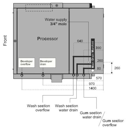
Prepare the installation site for water supply and drain connections according to the illustration. Please also refer to the "Space requirements" on page 12.
