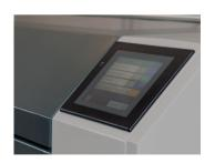
Operator friendly color touch screen with graphic display of all functions, 24 memory channels and PLC control.
