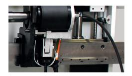
The maintenance free torque motor for positioning plates has an abolute position of  $\pm$  0,011 mm on a repeat of 580 mm. The motor contains no gears, minimising overall wear.
