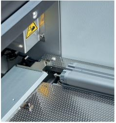
The updated pin bar loading system has fewer moving mechanical parts, which minimises the risk of plate infeed problems and improves serviceability.
