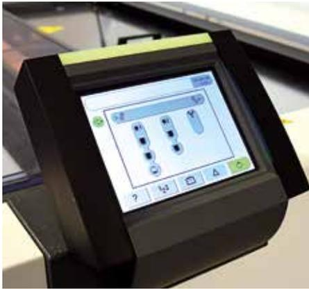
COU 85 HD is equipped with a full function touch screen display for easy operation and status monitoring.
