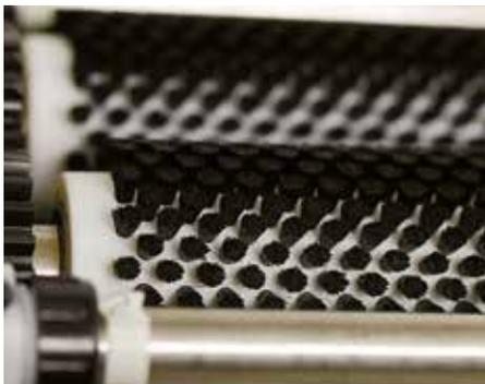
COU's are equipped with a double-brush configuration in the primary clean-out section. The COU 85 HD includes a second cleaning section with one brush offering improved plate cleaning and higher throughput.
