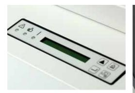
Gecko<sup>+</sup> has a simple control panel with status/ error information and function keys to quickly select between the four user-defined programs.
