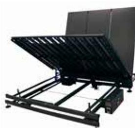
▲ The tipper flips the plate onto the trolley. Additional trolleys can be ordered.
