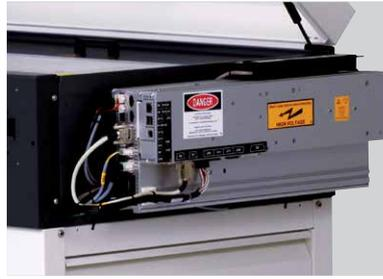
All electronics and mechanical components are located on the sides of the processor, for easy and convenient access during maintenance.
