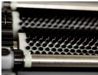
▲ Equipped with a double-brush configuration in the primary clean-out section.
