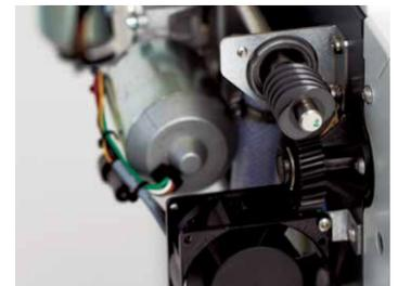
▲ The COU<sup>+</sup> uses a reliable and maintenance-free worm gear drive system to drive rollers and brushes.
