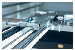
Advanced mechanics supported by servo controls provide accurate and reliable transport of the flexo plate through all processing steps.
