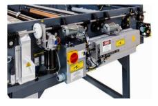
All electronics and mechanical components are located on the sides of the processor, for easy and convenient access during maintenance.
