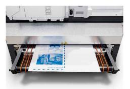
The imaged plates are manually fed through the integrated finishing unit which dries the plates and bonds the liquid dots to the plate surface.
